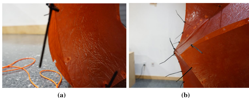
Fig. 13 Local failure (break off) (a), and local buckling of the fiberglass material (b)
