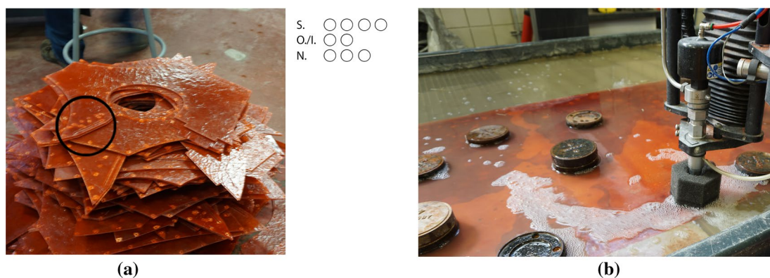
Fig. 11 Labeling system of assembly (a), and fabrication process (b) in waterjet cutting process
