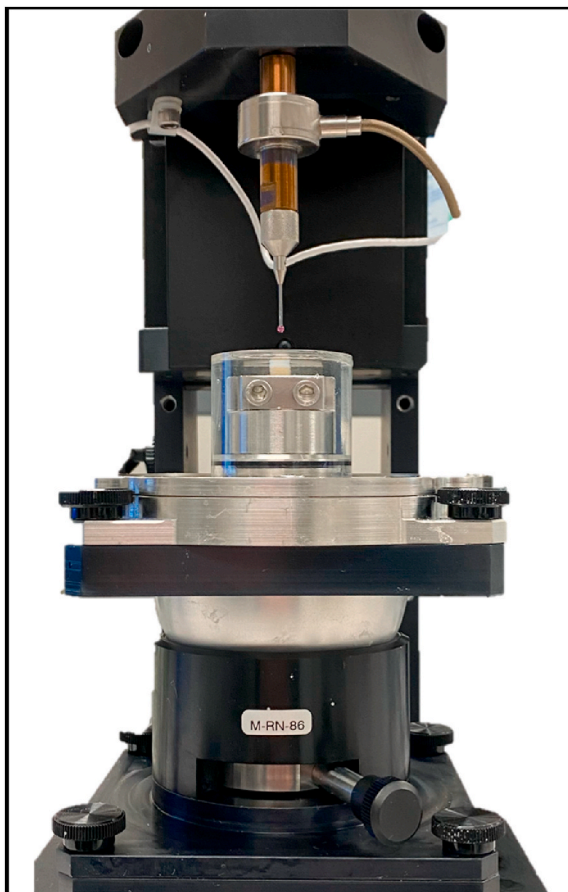
Fig. 2. Micromechanical tester, Mach-1 v500c (Biomomentum Inc.) used to perform indentation testing of cartilage samples.
